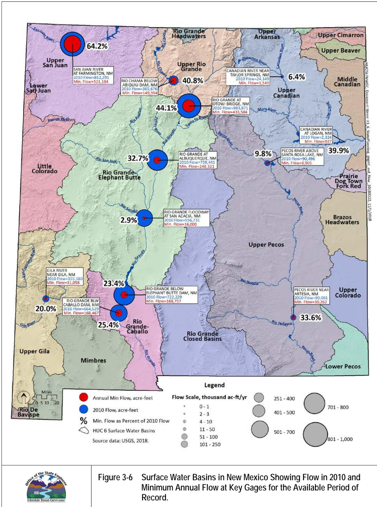
Figure 3-6 Surface Water Basins in New Mexico Showing Flow in 2010 and Minimum Annual Flow at Key Gages for the Available Period of Record.
